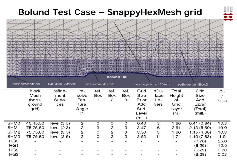
Table V. Bolund hill: Overview of different control parameters used to generate the SnappyHexMesh created grids. For definition ofdifferent parameters in the table - see tab. II. Positions of refinement boxes, surface layers and background grid is indicated in fig. 8.The SHM are SnappyHexMesh based grids and HG are HypGrid based ones.  $z_{0(L)} = z_{0-Land} = 0.015 \, \text{m}.$
